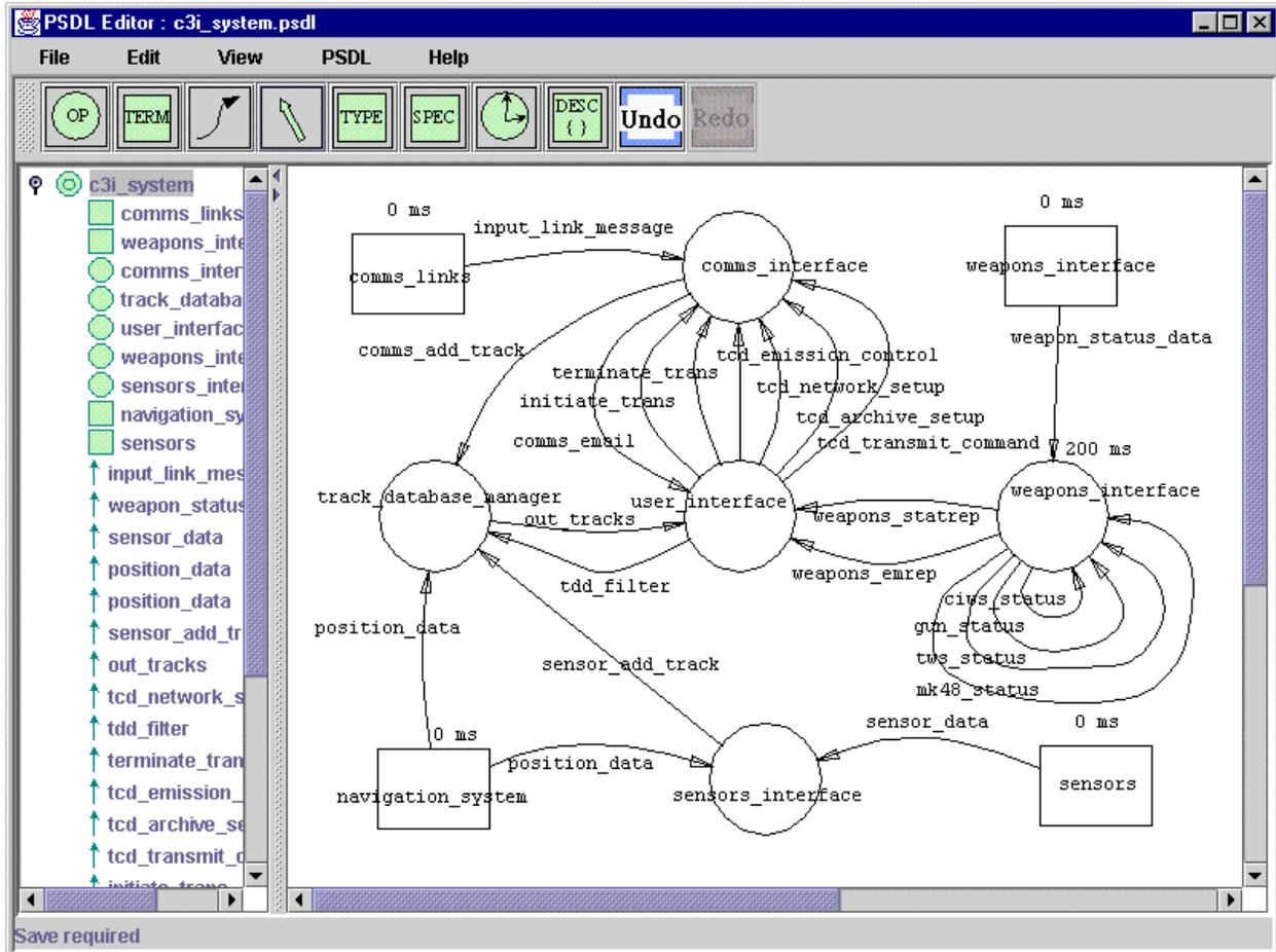
Figure 10. Top-level Dataflow Diagram of the c3i\_system.
