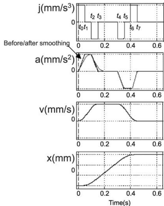
the trajectory generator. Second, the acceleration smoother is not located behind the sensor module or in the control loop. It is located inside the trajectory generator. So its implementation does not require redesign of the controller or robot.
