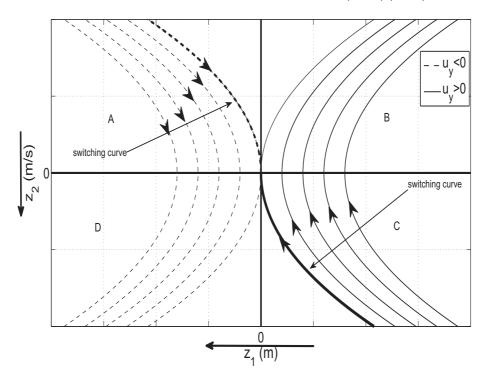
**Figure 5.1:** Qualitative shape of the curves on the phase plane of the double integrator subsystem  $(z_1 \text{ vs. } z_2)$  in case of constant thrust along the y axis for both the Hill-Clohessy-Wiltshire and the Schweighart-Sedwick models
