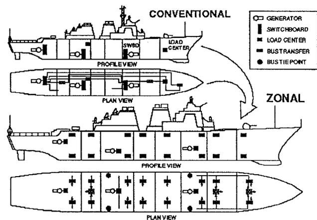
Fig. 1. DC Zonal Electric Distribution System (DC ZEDS)
