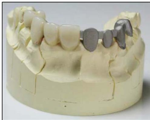
Figure 5. Dental Implants Made From CAD File Using DMLS (from Overton, 2009, p. 45)
