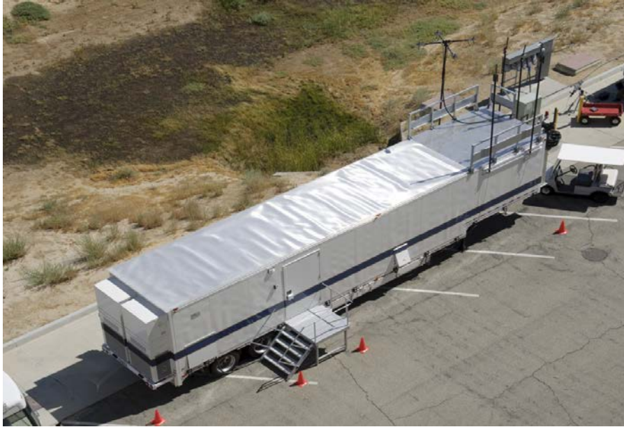
Figure 21. The NASA Global Hawk Mobile Operations Facility is a portable ground control station that can be transported anywhere for remote operations (from NASA/Tony Landis 2010. URL: http://www.nasa.gov/mission_pages/hurricanes/missions/hs3/news/pilot-challenges.html )
