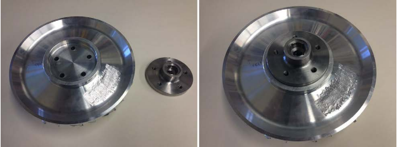
Figure 12. Rotor downstream face and new mounting flange
