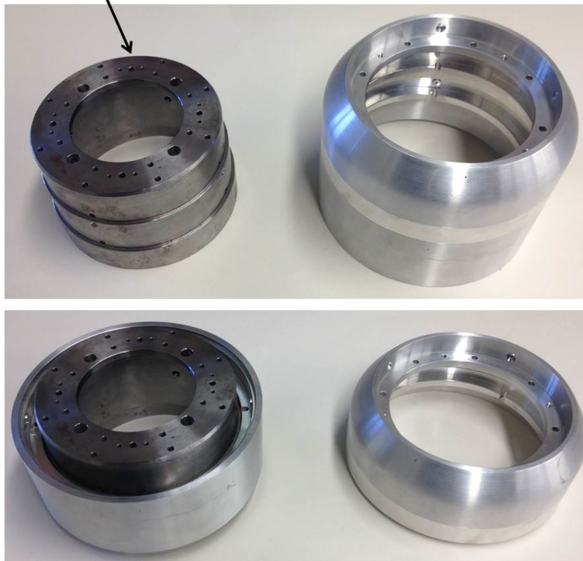
Figure 18. Stator Support Structure and “Blank” Stator Rings
