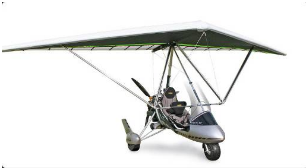
Figure 5. The XT912 Tundra Arrow. Made by Airborne in Australia. Engine: Rotax 912, 4 stroke 80HP. Speed: 65 Knots. Range: 700 KM (from Airborne, 2013).
