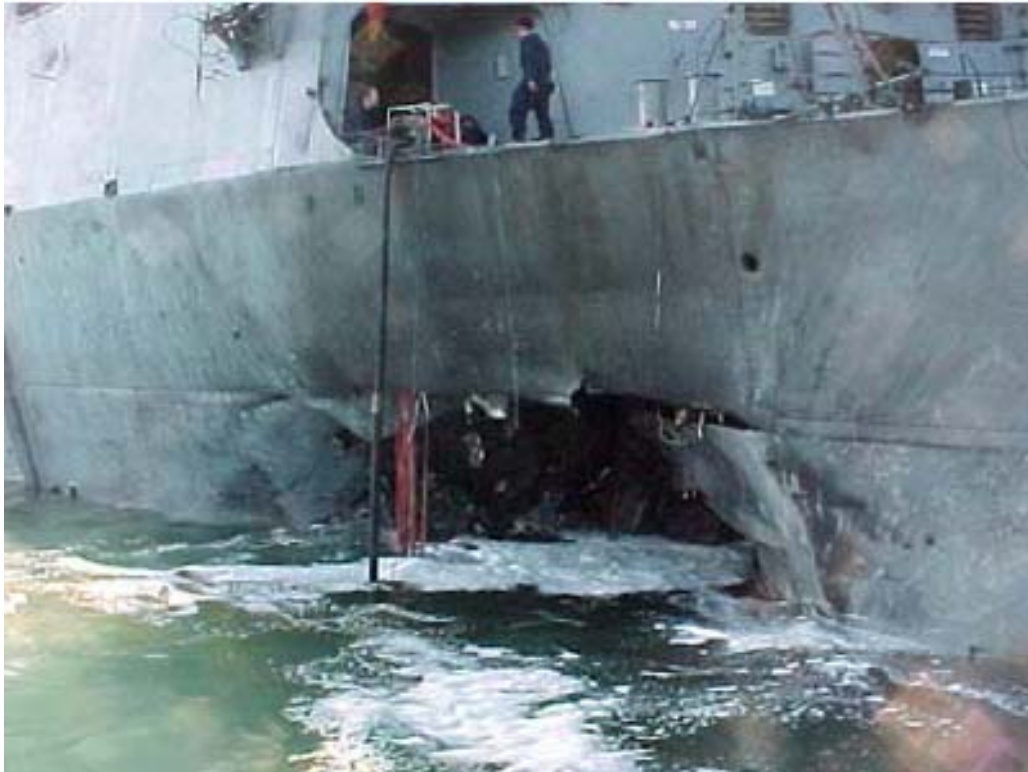
Figure 1. Damage to USS Cole from FIAC attack
