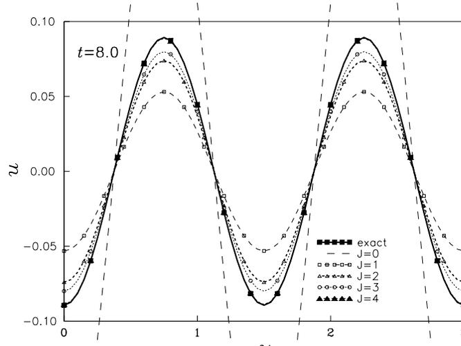
Figure 2. The non-dispersive wave-guide problem: comparison of solutions along the artificial boundary  $\mathcal{B}$ , at time  $t = 8$ .
