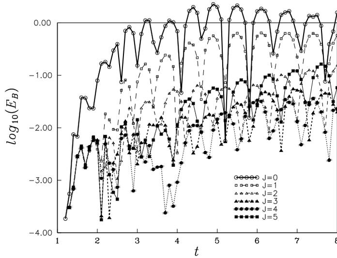
Figure 5. The dispersive wave-guide problem: global error  $E_B$  as a function of time for different values of the NRBC order  $J$ .
