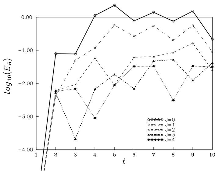
Figure 3. The non-dispersive wave-guide problem: global error  $E_B$  as a function of time for different values of the NRBC order  $J$ .
