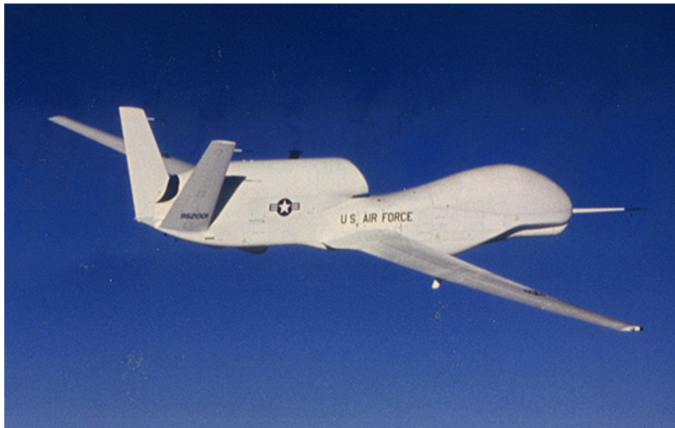
Figure 3. USAF RQ-4A Global Hawk high-altitude, long-endurance unmanned aerial reconnaissance system. (From: [15].)
