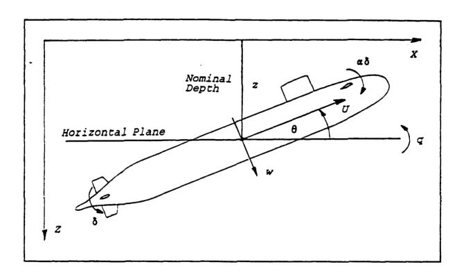
Figure (2.1) - Geometrical representations of the basic definitions for the equations of motion.
