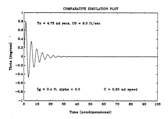
Figure (3.2) - An example of the stable response found in region I. This corresponds to Point a in fig. (3.1).
