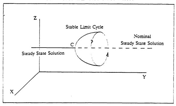
Figure (4.1) - An example of a supercritical Hopf bifurcation where the system has a nominal steady state solution until point C, which occurs at  $t_{\rm crit}$ . After  $t_{\rm crit}$  the system becomes unstable but forms a stable limit cycle.
