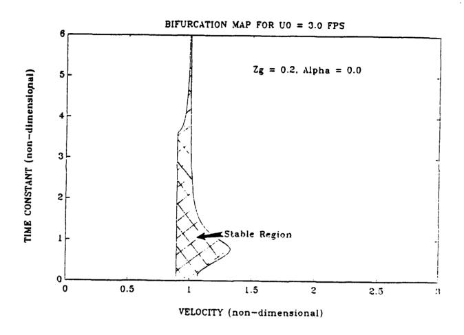
Figure (5.5) - This demonstrates the effects of an increase in the metacentric height for low nominal speeds.
