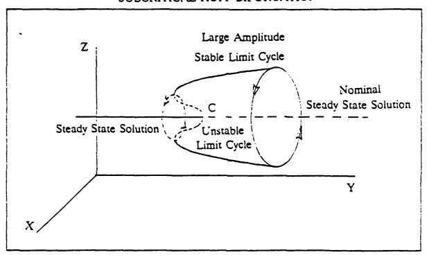
Figure (4.2) - This figure shows a subcritical Hopf bifurcation where the system loses stability prior to reaching point C, which again occurs at  $t_{\rm crit}$ .
