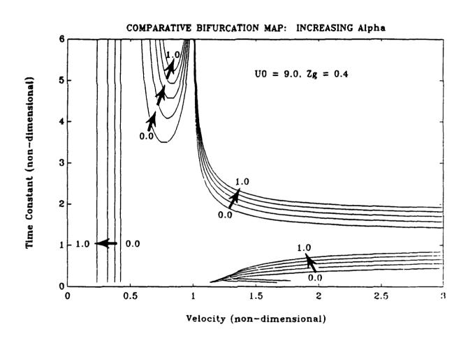
Figure (5.3) - The effects of changing the control surface gain coefficient,  $\alpha$ , on the bifurcation maps.
