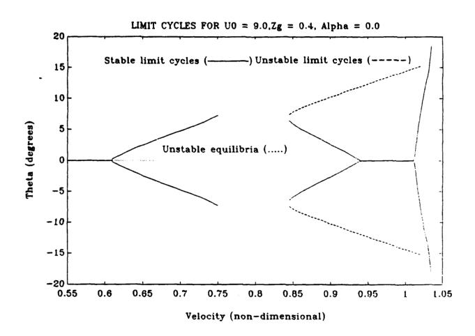
Figure (4.5) - This shows the amplitude response for a speed range encompassing the Hopf bifurcation points that are shown in fig. (3.1).
