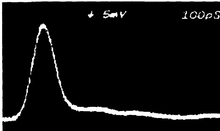
Figure A.1 Opto-Electronics Series PD-03 Photodetector response to 100 ps input pulse.
