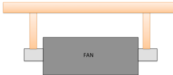
Figure 94: Rigidly Mounted Rotating System (Ex. Fan).
