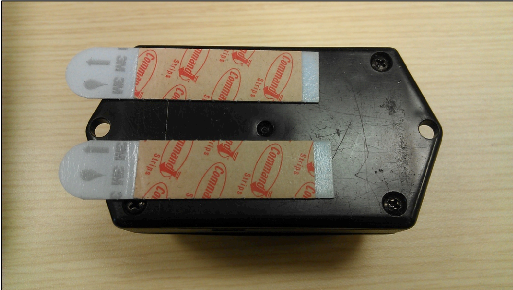
Figure 52: CAPTCHA Attaches to Equipment Via Command Strips.
