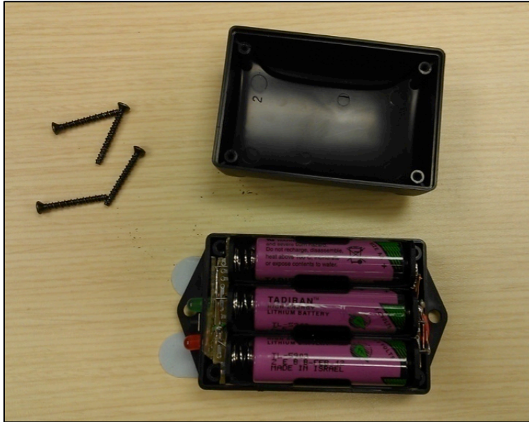
Figure 41: CAPTCHA Accelerometer with Triple Battery Power.
