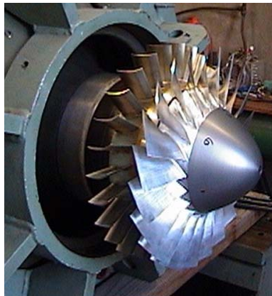
Figure 2. The transonic compressor rig at the Naval Postgraduate School
