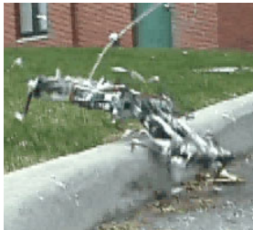
Figure 4: Whegs II flexing its body as it climbs over a curb
