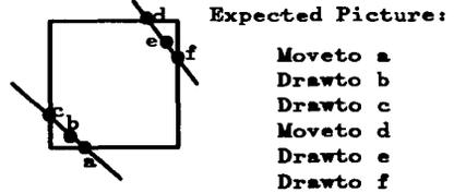
Case 7: One Contour Tangent, One Contour through Adjacent Edges
