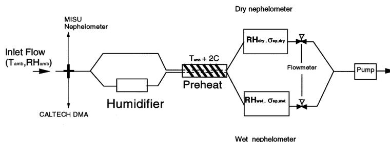
Fig. 1. Scheme of the University of Washington passive humidigraph.
