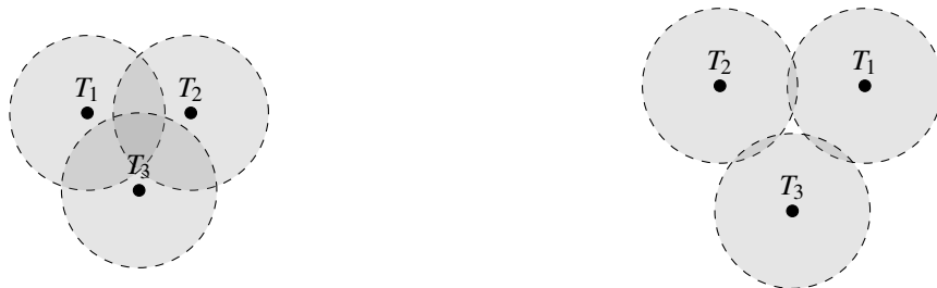
Figure 2.7: Clusters Special Case - The targets in the left plot form exactly one cluster. The targets on the right, however, form the three clusters \{T_1, T_2\} , \{T_2, T_3\} and \{T_1, T_3\} since the three targets do not have a single point in common.
