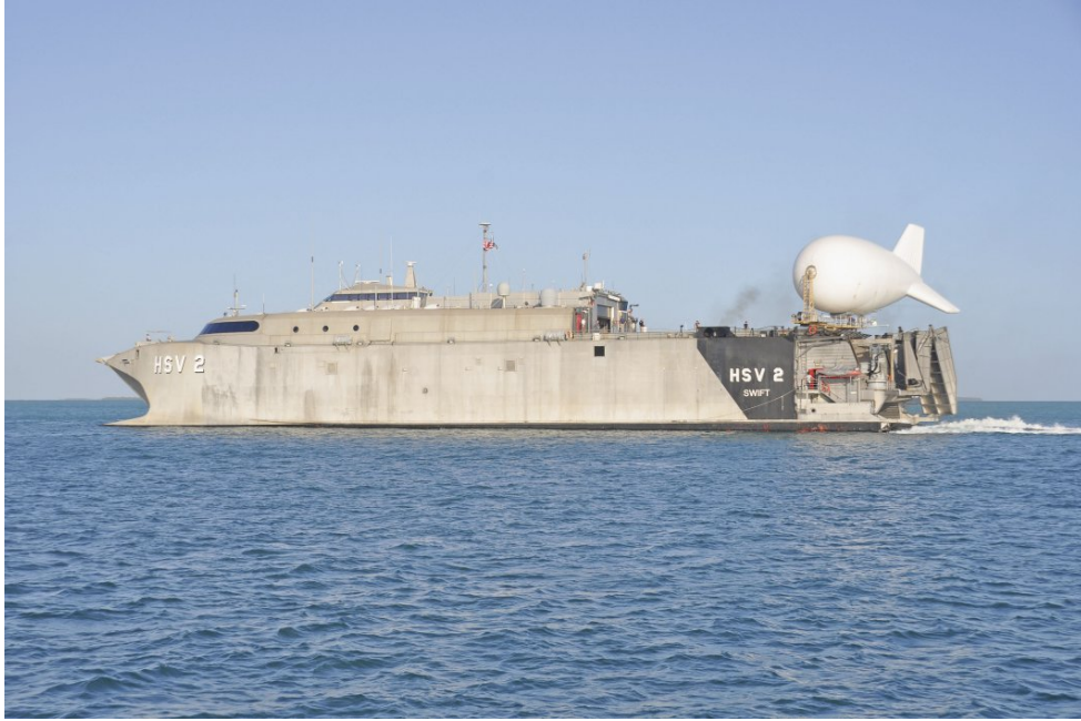
Figure 10. Aerostat operating from USNS SWIFT (HSV 2) (from Wasserbly 2013).
