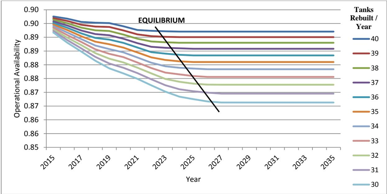
Figure 7. USMC M1A1 Forecasted A<sub>0</sub> Through 2035 by Rebuild Level
