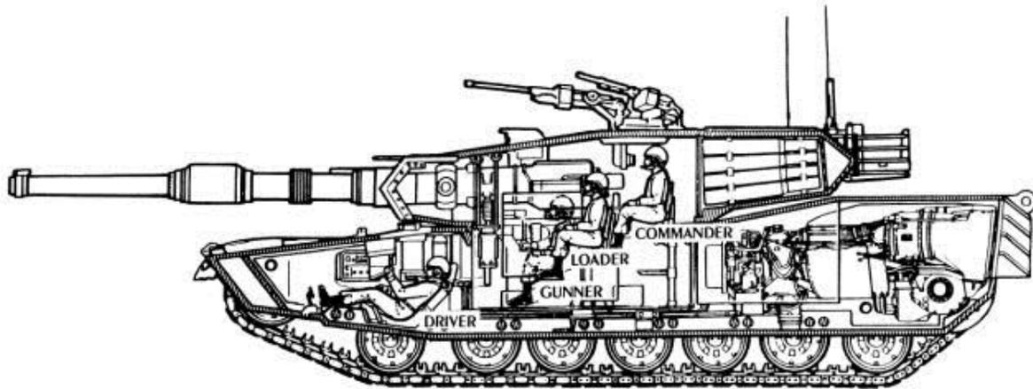
Figure 1. Cutaway Drawing of M1A1 MBT Showing Position of Main Components (from Jane's Information Group, 2013)
