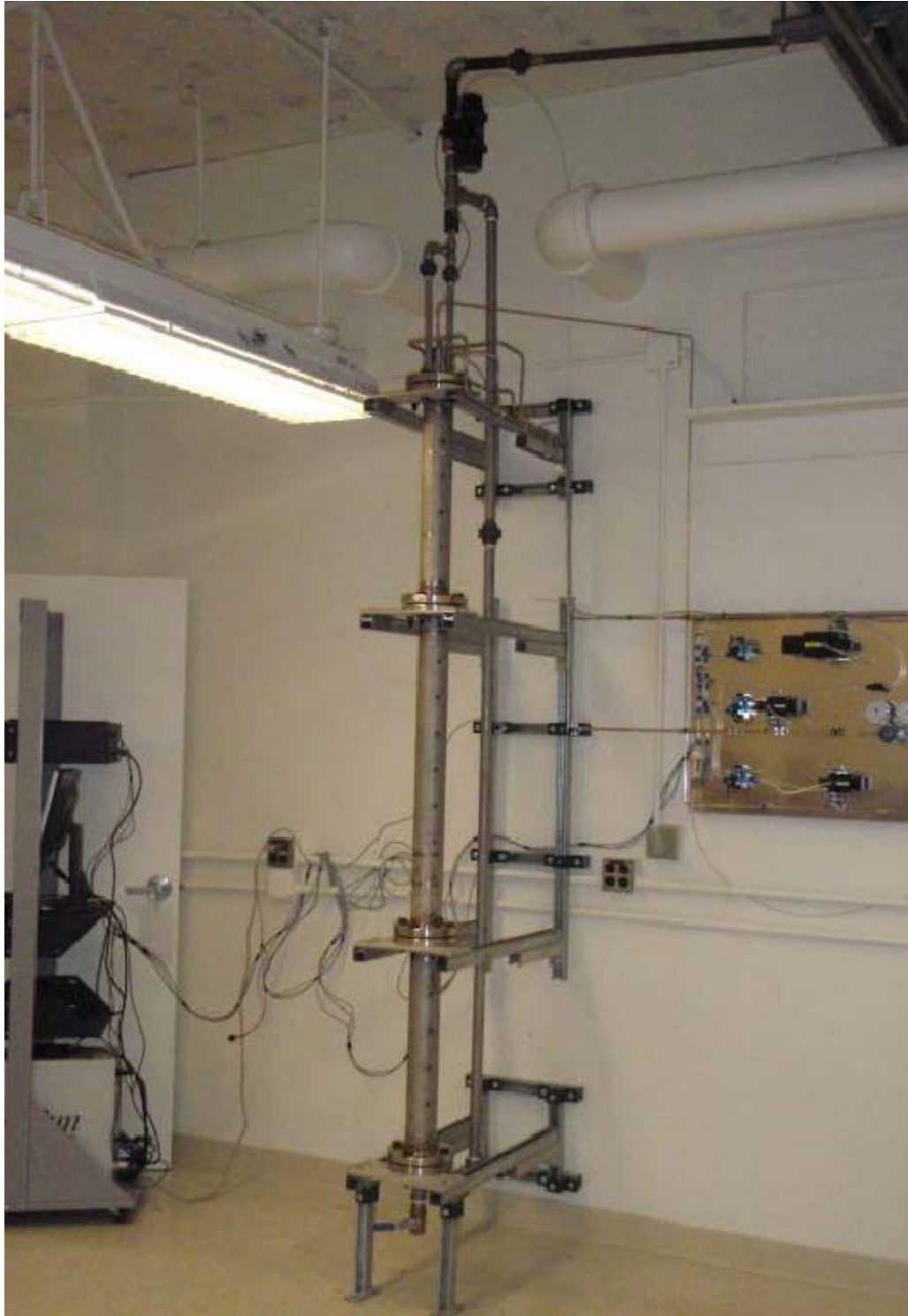
Figure 1. The Combustion Chamber
