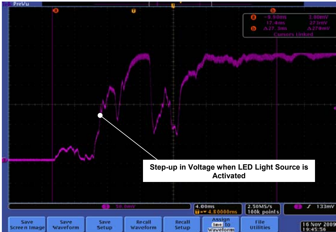
Figure 30. Signal Reading from Oscilloscope during Testing
