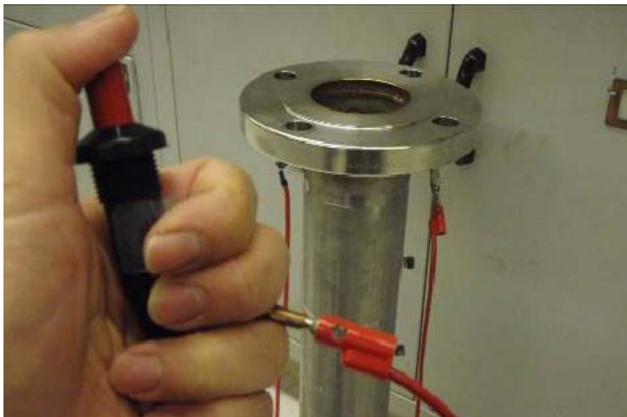
Figure 32. Piezoelectric Igniter used for the Generation of Sparks
