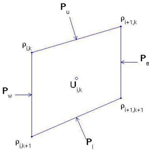
Figure 2. Double finite-volumes for C-grid.
