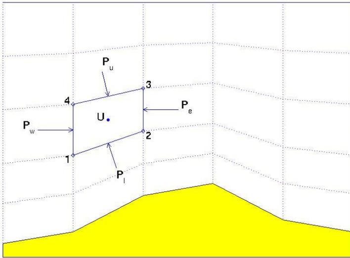
Figure 1. Finite-volume discretization and staggered grid in terrain-following coordinates with two cells representing  $r > 1$  and  $r < 1$ .
