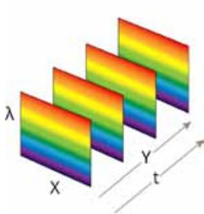
Figure 1: A pushbroom imager collects complete spectral and spatial data over time, for every pixel within the field of view. This is the essential difference between multispectral and hyperspectral
