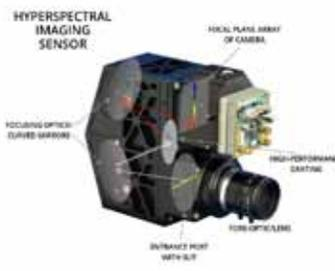
Figure 3: Headwall’s Micro-Hyperspec sensor is designed for airborne applications where low weight and small size are key requirements. The all-reflective concentric design provides high spatial and spectral resolution, high SNR, low stray light, and aberration-corrected imaging.
