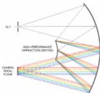
Figure 2: All-reflective, concentric imager using high-performance diffraction grating and concave mirrors yields an elegant, simple, and high-performance hyperspectral sensor.
