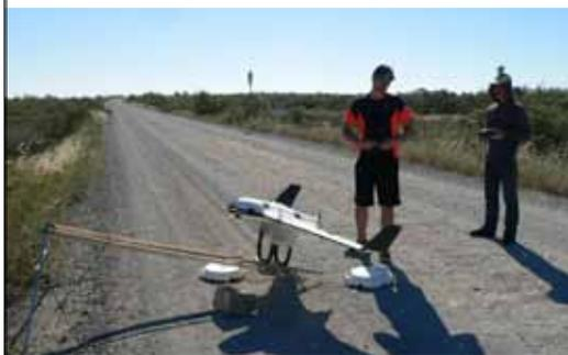
An X8 Flying Wing UAV being launched from land to look down at floating tags in the coastal ocean
