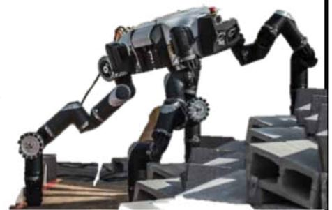
NASA-JPL's RoboSimian climbing over an obstacle simulating a rubble pile. This technology is being examined for autonomous maritime mobile manipulation tasks by ONR-RC.
