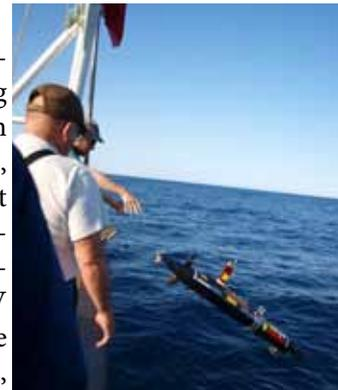
UPorto Xplorer AUV hand-launched from the support vessel for tracking *Mola mola*
