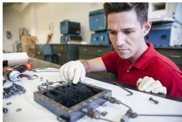
Lt. Will Curtin, a student in the mechanical engineering program, demonstrates the carbon nano-fiber foam (CFF) following its creation in the NPS Functional Materials Laboratory. For the first time, NPS researchers have developed a CFF that behaves as a viscoelastic solid with stable mechanical properties without the need of a polymeric component.
