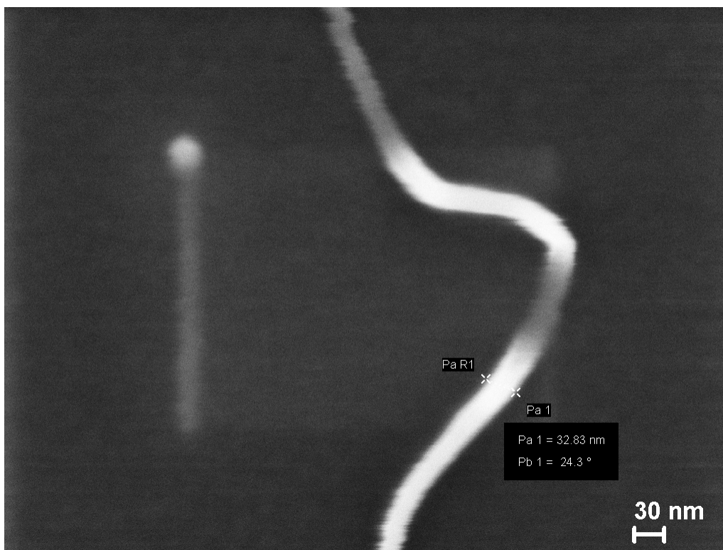
Figure 8. Straight Surface of Pristine Nanotube
