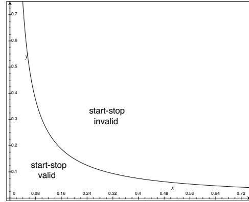
Fig. 1. This shows the region of validity for the start-stop approximation for X-band (wavelength 3cm). The horizontal axis represents the waveform duration, and the vertical axis shows the relative velocity. For shorter wavelengths, the curve moves towards the axes, and the region of validity is smaller.
