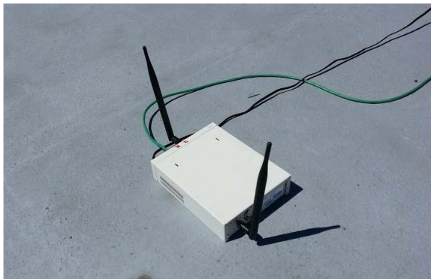
Figure 20. Cognitive radio station using two separated transmitter and receiver antennas.
