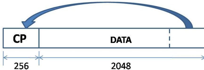
Figure 14. Example of cyclic prefix (CP) in OFDM modulation (from [28]).
