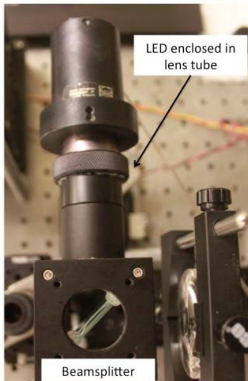
Figure 9. Top view of the self-aligned collimated LED assembly. The LED point source was enclosed in a lens tube produce a collimated output. The beam splitter reflects the collimated light onto the MEMS detector and the reflected light from the MEMS detector is then transmitted through the beamsplitter to the Fourier 4F optical system.
