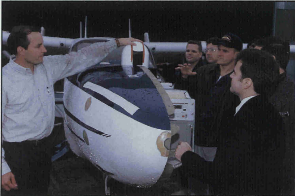
Meteorology Professor Phil Durkee (left) explains the function of a solar sunphotometer, a device that measures optical range, to some of his students. The meter is mounted on the nose of NPS's Pelican unmanned aerial vehicle.
