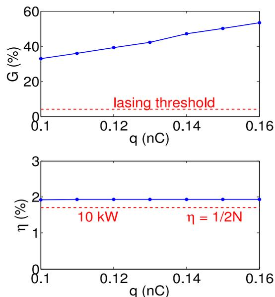
Figure 1: Weak-field gain  $G$  and steady-state extraction  $\eta$  versus electron bunch charge  $q$ . The gain increases linearly with  $q$ , while the extraction is constant. The minimum gain for lasing and the minimum extraction to achieve 10 kW output power are indicated by dashed red lines.
