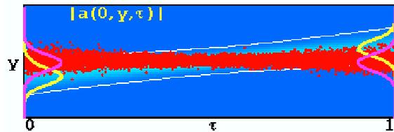
Figure 7: Simulation output showing a cross-section of the optical mode  $|a(y, \tau)|$  over a single pass through the undulator, with red dots representing sample electrons, for an output mirror tilt of  $\theta_m = 6 \mu\text{rad}$ . The yellow curves depict the optical mode profile  $|a(y)|$  at the beginning ( $\tau = 0$ ) and end ( $\tau = 1$ ) of the undulator, and the purple curves depict the fundamental mode profile for no mirror tilt.
