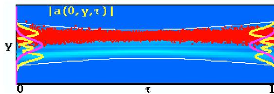
Figure 9: Simulation output showing a cross-section of the optical field amplitude  $|a(y, \tau)|$  over a single pass through the undulator, with red dots representing sample electrons, for an electron beam shifted off-axis 0.9 mm. Note the presence of higher-order modes in the yellow curves, which depict the optical mode profile  $|a(y)|$  at each end of the undulator.
