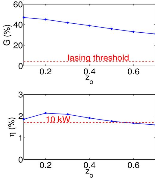
Figure 5: Weak-field gain  $G$  and steady-state extraction  $\eta$  versus normalized Rayleigh length,  $z_0 = Z_0/L$ . The gain increases as the Rayleigh length decreases; the optimum extraction is at  $z_0 \approx 0.2$ .
