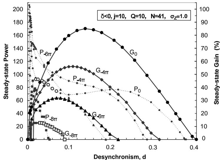
Fig. 4. Steady-state, saturated power  $P$  and weak-field, steady-state gain  $G$  versus desynchronism for negative taper rates  $\delta = 0, -4\pi, -6\pi$ , and  $-8\pi$ .
