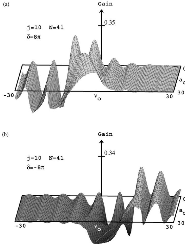
Fig. 1. FEL gain spectrum  $G(v_0, a_0)$  for large tapers. (a)  $\delta = +8\pi$ ; (b)  $\delta = -8\pi$ .
