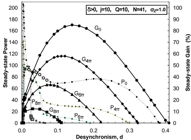
Fig. 3. Steady-state, saturated power  $P$  and weak-field, steady-state gain  $G$  versus desynchronism for positive taper rates  $\delta = 0, +4\pi, +6\pi$ , and  $+8\pi$ .
