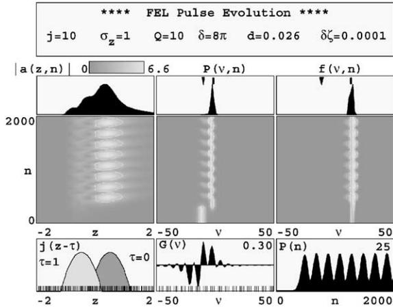
Fig. 2. Multimode simulation for  $j = 10$ ,  $d = 0.026$ , and  $\delta = +8\pi$ . The various quantities are explained in the text. In this case, the oscillations in  $|a(z, n)|$ ,  $P(v, n)$ ,  $f(v, n)$ , and  $P(n)$  are evidence for limit-cycle behavior.
