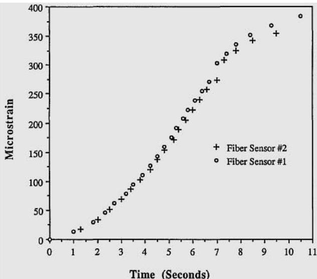
Fig. 3. Data processor output showing the variation of strain versus time. Typical output waveforms shown in Fig. 2 were fed into a software package to acquire strain information at each instant in time.
