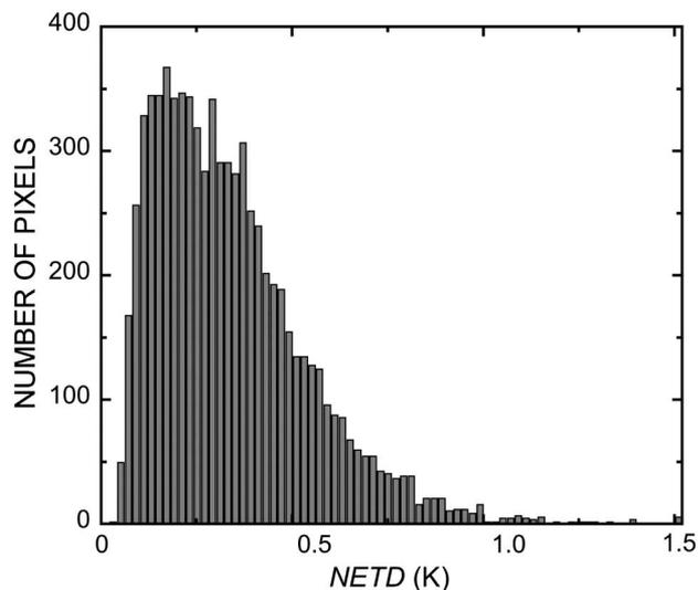
Fig. 3. NETD histograms show that the peak number of individual detector elements exhibit NETD values of less than 200 mK, with some devices showing less than 50 mK.
