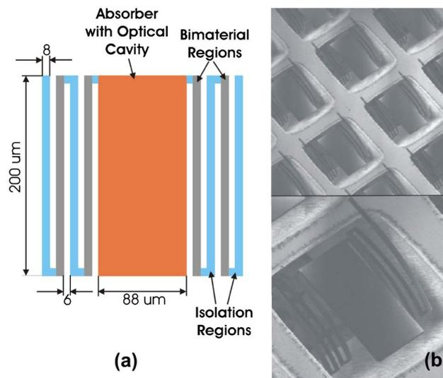
Fig. 1. (Color online) (a) Multifold structure was chosen in order to increase the effective lengths of both thermal isolation and bimaterial regions without increasing the overall detector size. (b) Micrograph images showing a single detector and part of the array.
