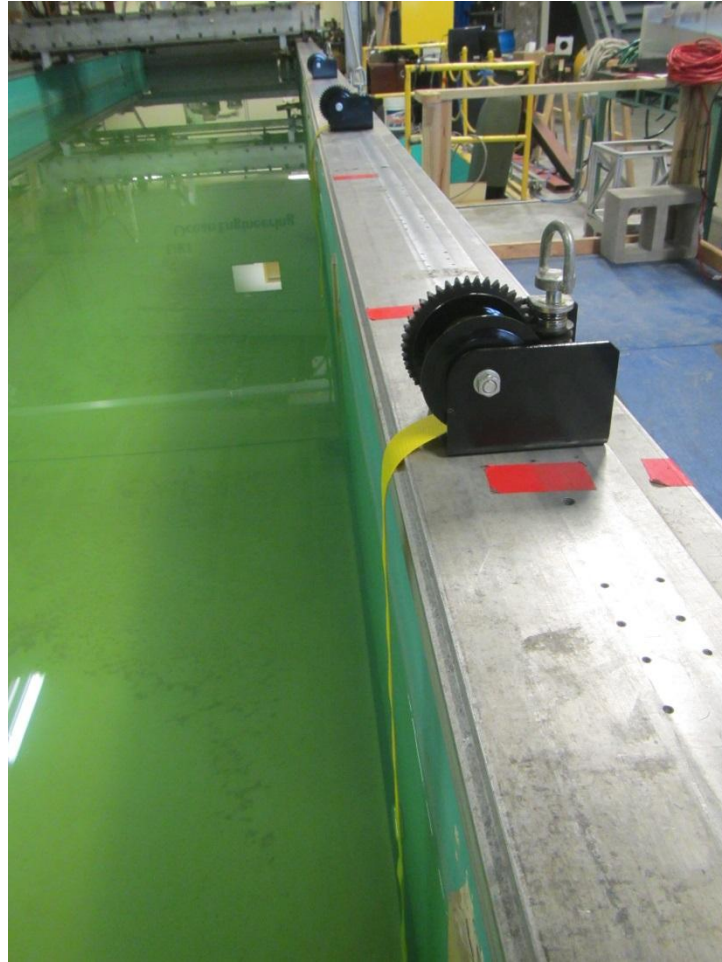
Figure 23. Winches ready to move the metal plate seams of the beach
