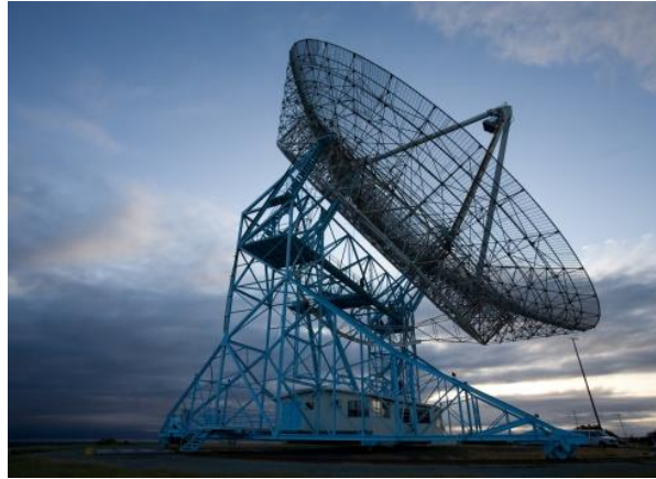
Figure 4. A 150-foot satellite dish antenna in Stanford, California. SRI International (from http://www.sri.com/research-development/specialized-facilities/dish-radio-antenna-facility , November 3, 2014)
