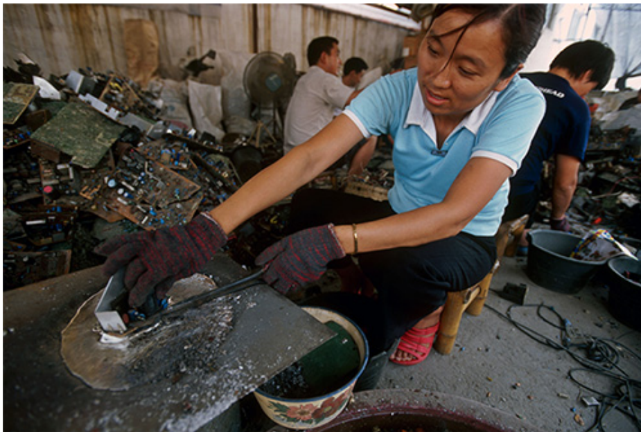
Figure 4. A woman in Taizhou, China, melts a circuit board to remove the metal chips (Basel Action Network, 2007)
