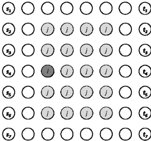
Figure 3. Network topology used in this thesis (we call this the “long-arc topology”). Nodes are laid out in a regular, square grid, with each node  $i$  connected by directed arcs  $(i, j)$  to neighbor nodes  $j$ , as shown. For simplicity, no arcs are shown.
