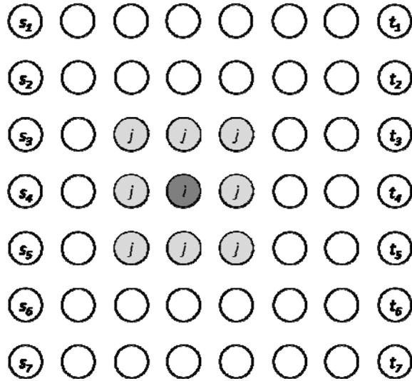
Figure 2. Network topology used by Bekker and Schmid (2006). They use a regular, square grid of nodes and connect each node  $i$  to each of its nearest neighbors  $j$ , using a directed arc  $(i, j)$ . Note that “nearest neighbors” includes nodes that are diagonally adjacent. For simplicity, no arcs are shown.
