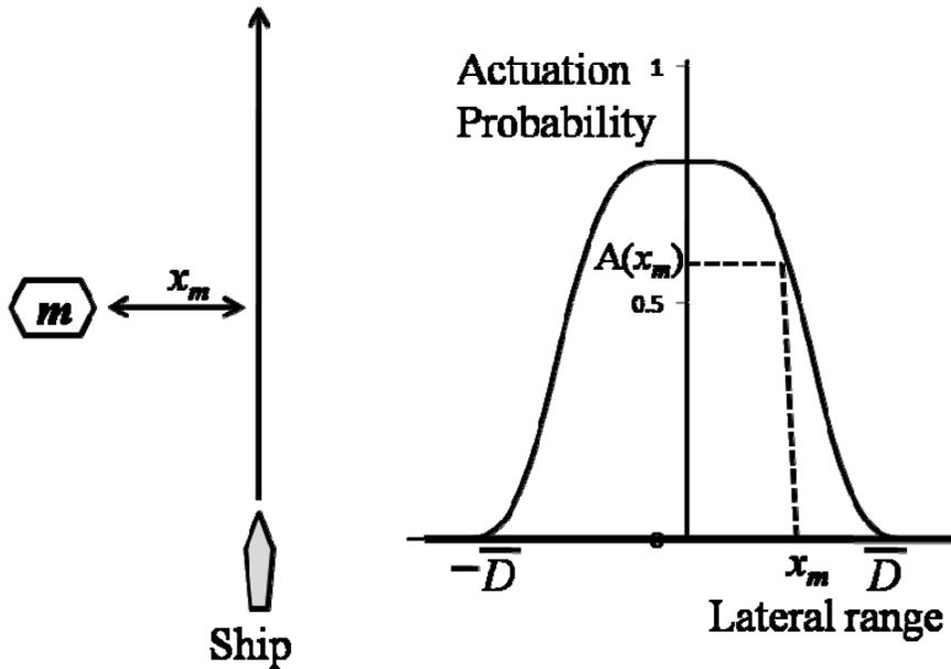
Figure 5. Actuation curves. When a ship transits along a straight path, infinite in both directions, and with CPA  $x_m$  (lateral range) to a mine  $m$ , then the probability of mine actuation during the transit is  $A(x_m)$ .
