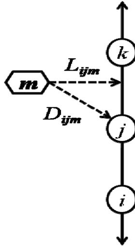
Figure 6. Definition of  $D_{ijm}$  and  $L_{ijm}$ .  $D_{ijm}$  is the CPA distance from mine  $m$  to arc  $(i, j)$ , while  $L_{ijm}$  is the CPA distance from mine  $m$  to arc  $(i, j)$  extended in both directions to edge of Q route.
