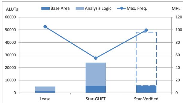
Figure 8: Area and Frequency comparison among secure CPUs.
