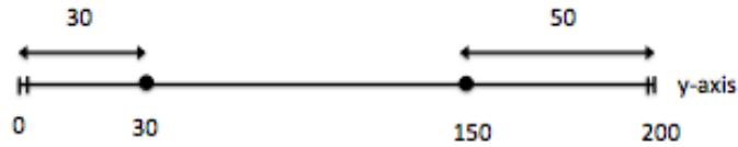
Figure 4.3: Visualization of the base locations and the distances from the edges for the two-base example where bases are at y=30 and y=150 respectively
