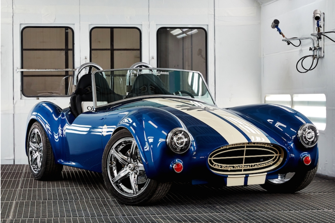
Figure 6. Replica Shelby Cobra printed by ORNL (from Oak Ridge National Laboratory, http://web.ornl.gov/sci/manufacturing/media/news/detroit-show/ )
