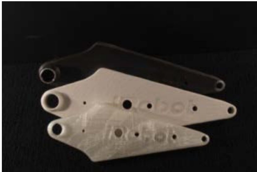
Figure 7. Printed lightweight flippers for PackBot (from Zunino, 2014)
