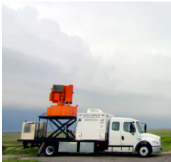
Figure 1. MWR-05XP in the Texas Panhandle on 21 May 2007 scanning an approaching squall line. View is to the northwest. Photograph © H. Bluestein.
