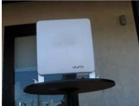
Figure 5. Phased array base station at USCG Station, Monterey Bay.
