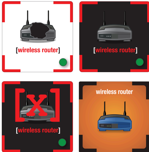
Figure 1: Early designs for a compromised node: a physical “hole” in a greyed-out icon (top left), a negated color change (top right), an X and a negated color change (bottom left), and the final design (bottom right) using just a background color change.
