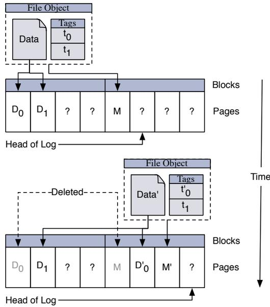
Fig. 3: A page-level view of a file being updated. In this example, the first logical page of the file is updated. This results in the replacement of the prior tag ( $t_0$ ) with a new tag ( $t'_0$ ), effectively deleting the prior version of the data page ( $D_0$ ). A new file object is re-written ( $M'$ ) and a new tag for that object is stored in its parent object, effectively deleting the previous object ( $M$ ).
