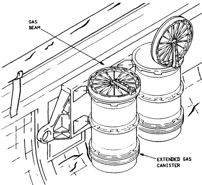
Fig. 4 Extended GAS Canister Mounted in Shuttle Bay
