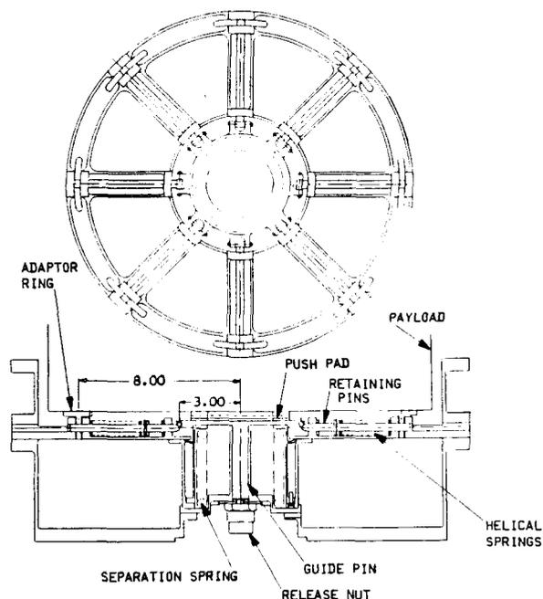
Fig. 2 GAS Canister Extension and Launch Mechanism Cross Section
