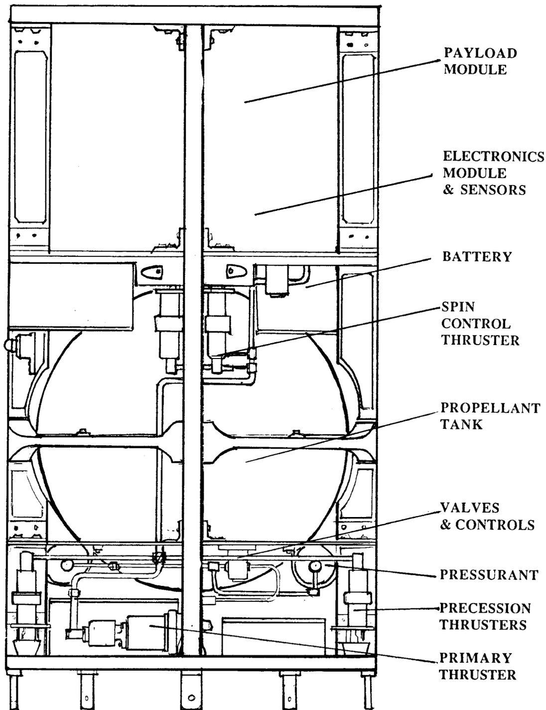
Fig. 6 Cross Section of ORION General Purpose Satellite
