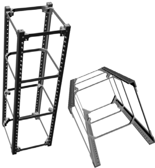
Figure 1: CNGB structure showed with end-feet crossbar removed on the right.
