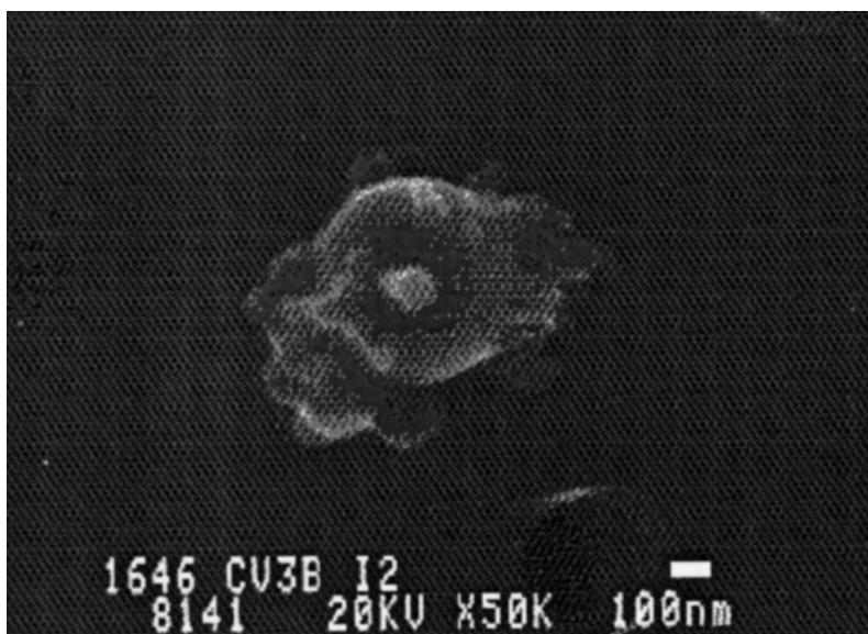
FIG. 2. Scanning electron microscope image of a combustion-derived particle collected in the USS Mount Vernon plume on 27 Jun.
